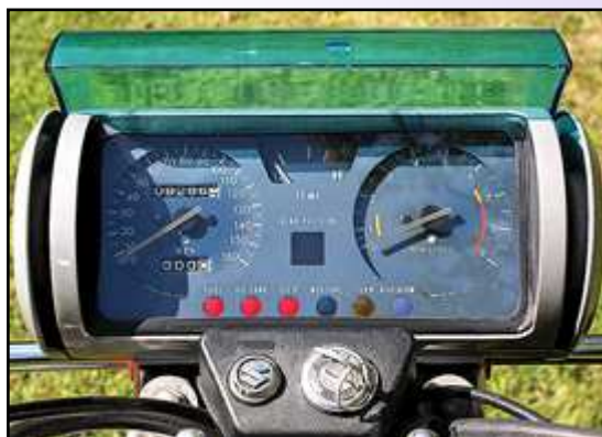
Distinctive Suzuki RE5 gauge cluster cover pops open when the key is turned to ON. Note the digital gear position indicator.
