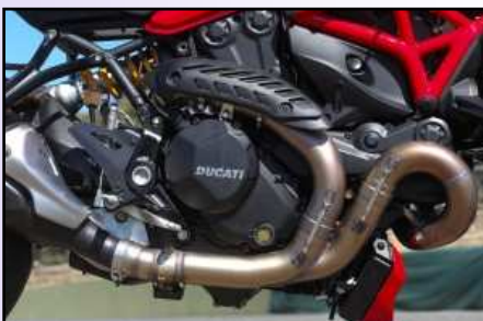
Larger throttle bodies, higher compression and a new exhaust system boost output to 160 horsepower and 97 lb-ft of torque.
