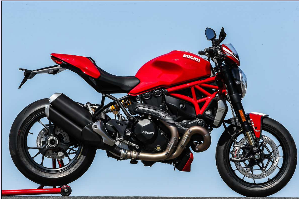
The 2016 Ducati Monster 1200 R has fully adjustable Öhlins suspension, Brembo brakes and forged Marchesini wheels.
