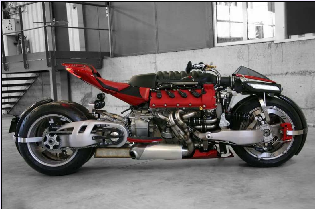
Lazareth LM 847: twin chain drive at the rear end (Credit: Lazareth)
