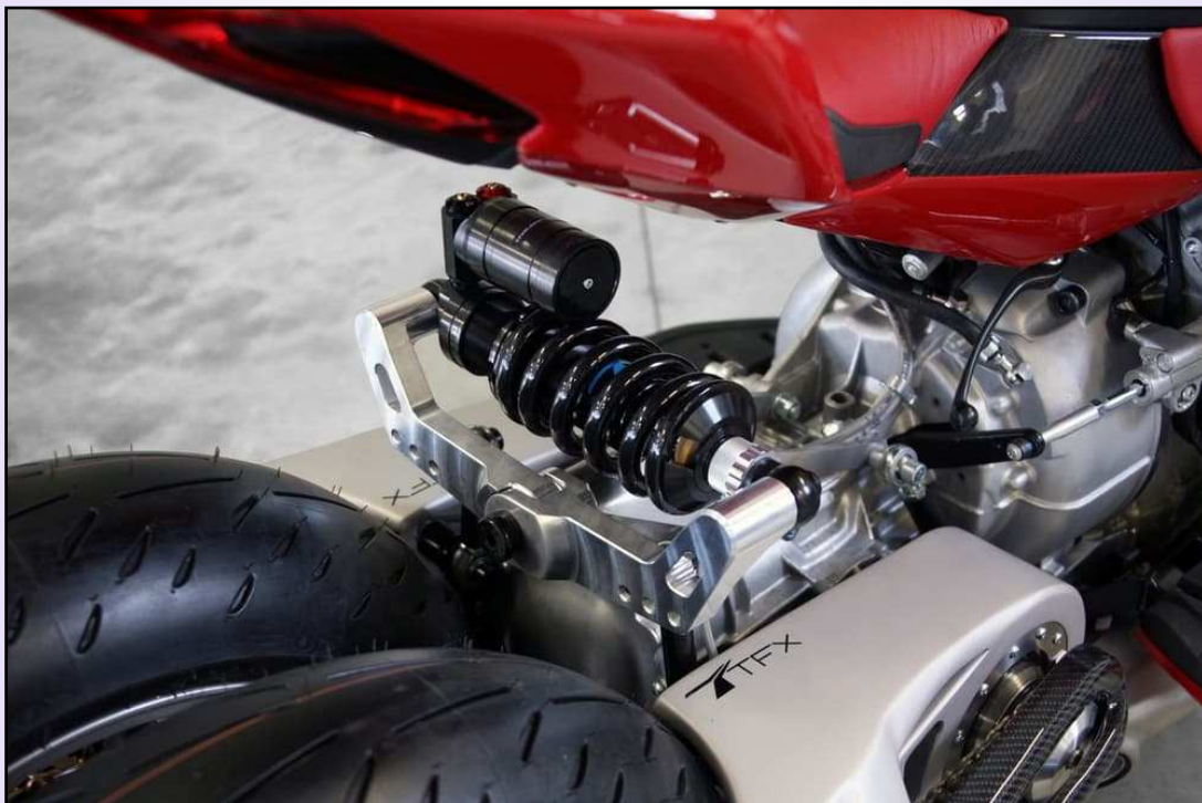
Lazareth LM 847: odd rear suspension arrangement seems to damp both regular suspension motion and any motion that would move one wheel independently of the other - for example, cornering lean angle changes (Credit: Lazareth)
