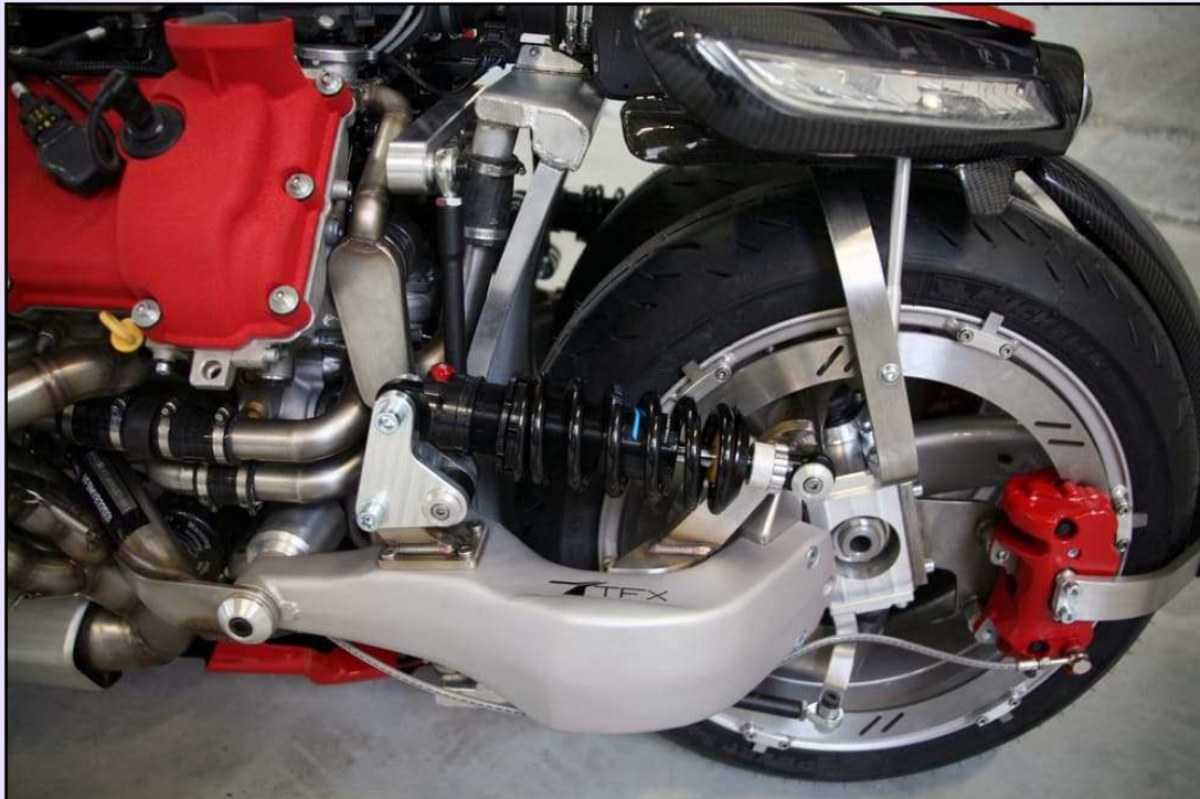
Lazareth LM 847: front right swing arm with independent shock and rim-mounted brake disc (Credit: Lazareth)
