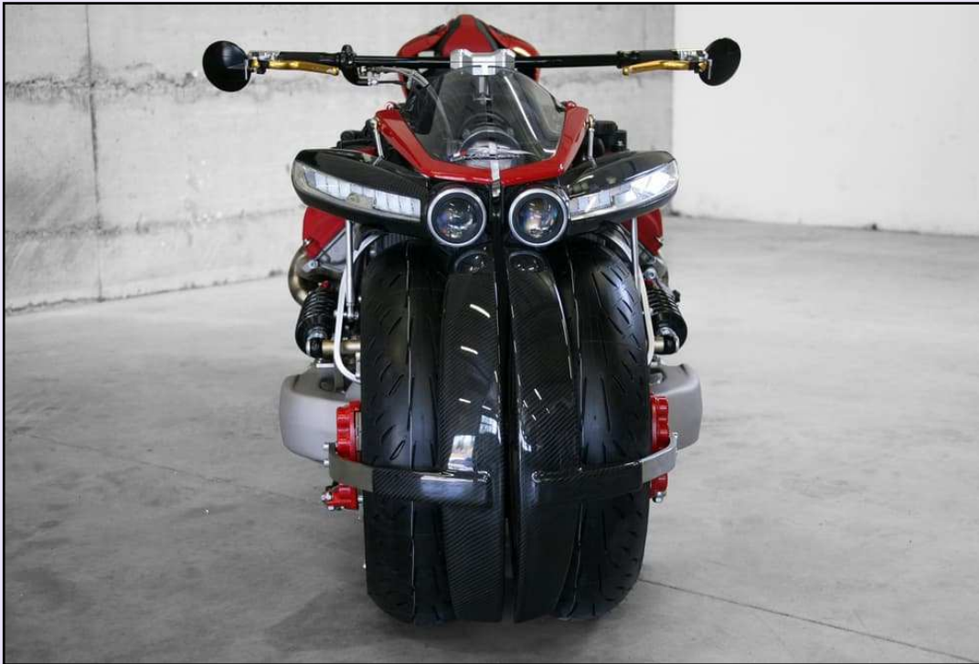
Lazareth LM 847: carbon aero fairings in front of the wheels (Credit: Lazareth)
