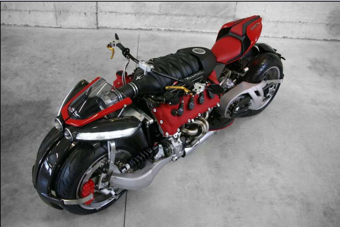
Lazareth LM 847: rider is draped over a 4.7-liter Maserati/Ferrari engine (Credit: Lazareth)
