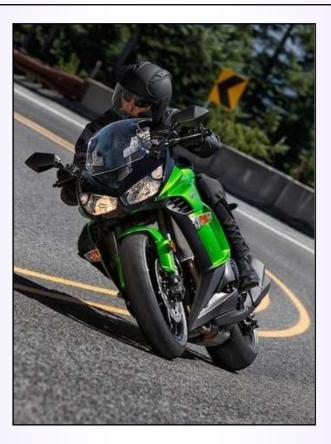
If you are too stiff on your bike, your body movements can also have undesirable steering inputs. These front-end shakes will transfer through your whole body, which will act as extra inertia on the steering system reducing the bikes self-aligning effect and turning performance.
