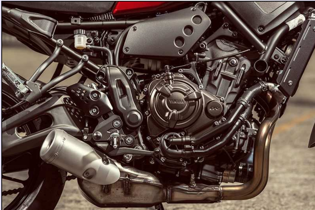
The liquid-cooled, fuel-injected 689cc Crossplane Concept parallel twin makes a claimed 50 lb-ft of torque.
