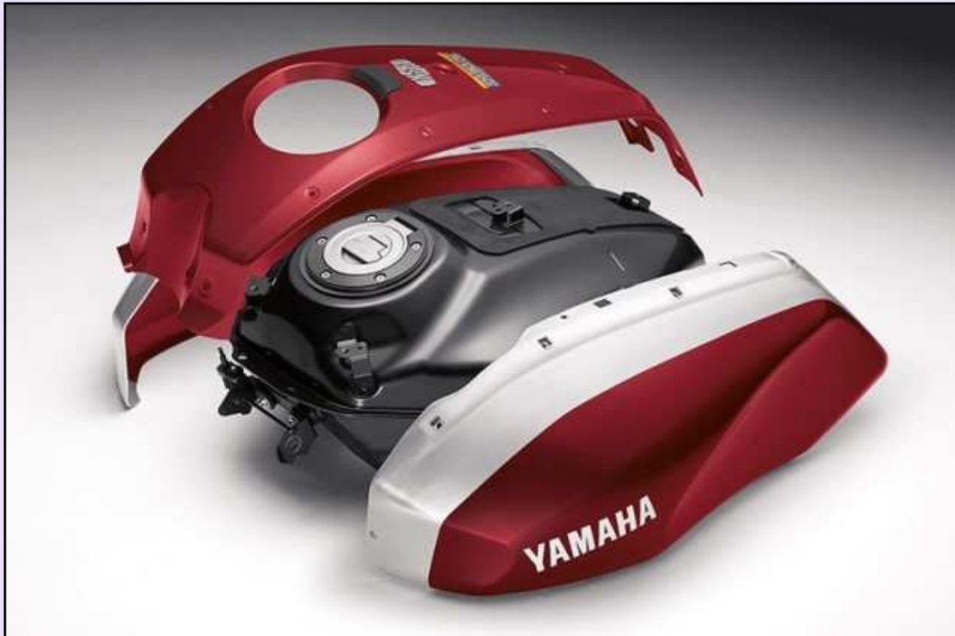
The Yamaha XSR700's aluminium tank panels are removable for easy customization.
