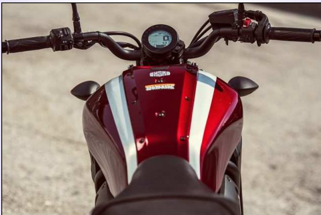
The 2018 Yamaha XSR700 has a taller, wider handlebar and all-LCD meter.
