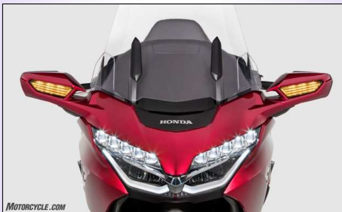
For 2018, all Gold Wing lighting is now from LEDs. Look to the mirror mounts and the lower edge of the windscreen to see the new airflow ducts.
