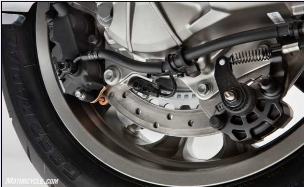
The single piston caliper (right) is the parking brake for the DCT models and is actuated by a lever on the lower left side of the fairing.
