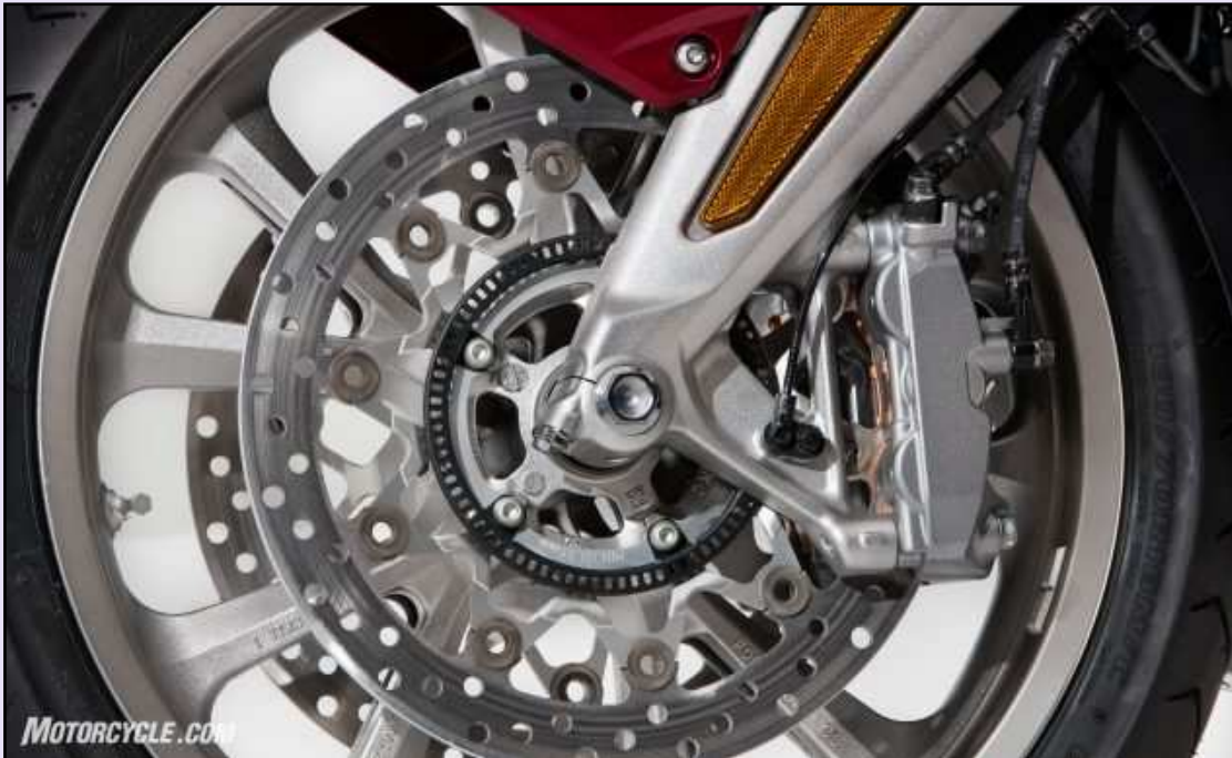
Honda's combined ABS slows the front end with a pair of six-piston radially-mounted calipers squeezing 320mm rotors.
