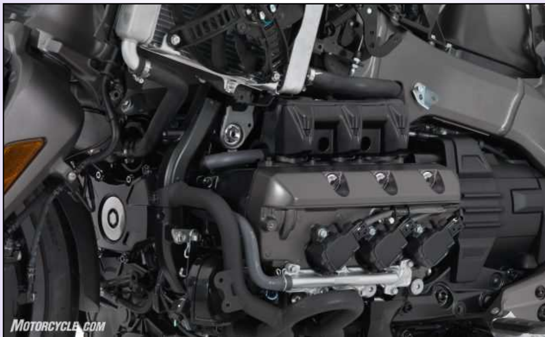
The new engine is 29mm shorter front-to-back which allows it to be moved further forward in the frame.
