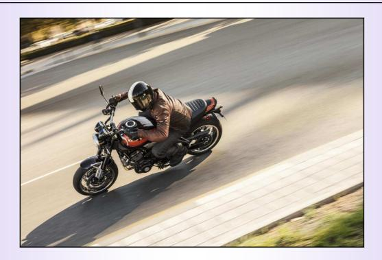
Like the Z1, the Z900RS features a 948cc-class inline four – an engine configuration that inherently offers a great balance of power and manageability. Tuning focuses on the low-mid range. Revs build in a measured, but very determined manner, giving the rider a sense of connectedness between the throttle and rear wheel.
