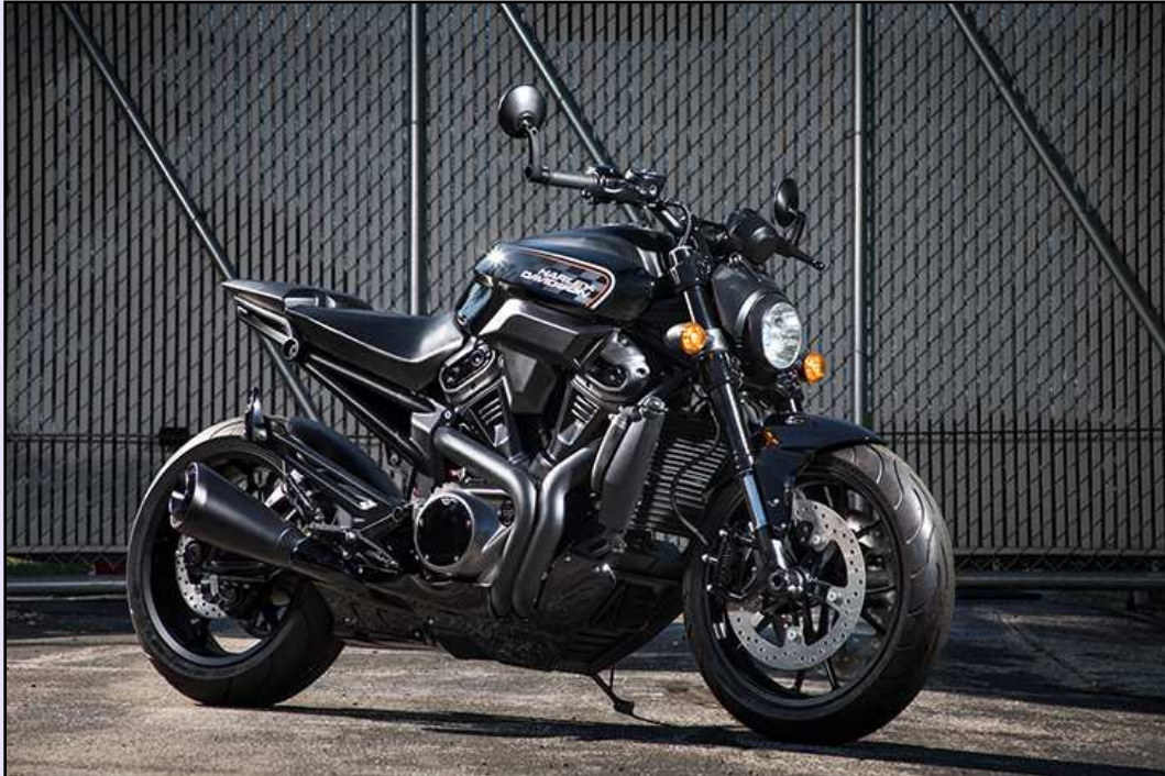
This 975cc Streetfighter model is part of Harley-Davidson's new modular 500cc to 1250cc middleweight platform of motorcycles, which is planned to launch in 2020. (Prototype model shown)
