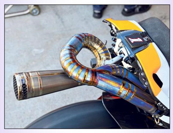
"One additional benefit of titanium is its corrosion resistance. Titanium is so reactive with the oxygen in the air that it forms a microscopic oxide layer on its surface which protects it from further attack.
