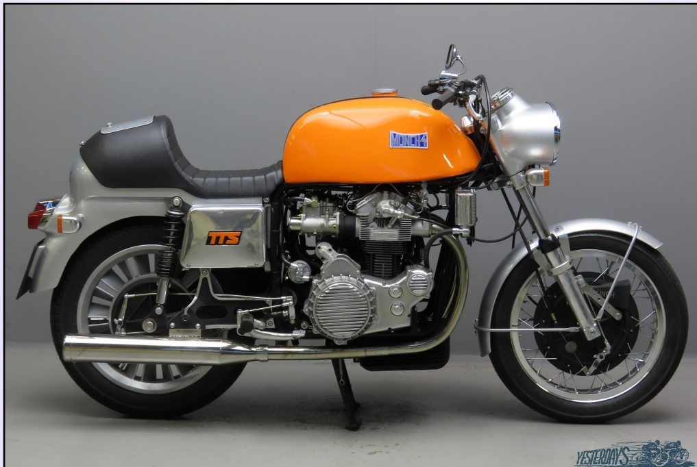
Münch 1973 Mammut TTS Recreation 1200cc NSU OHC four cylinder frame & engine
