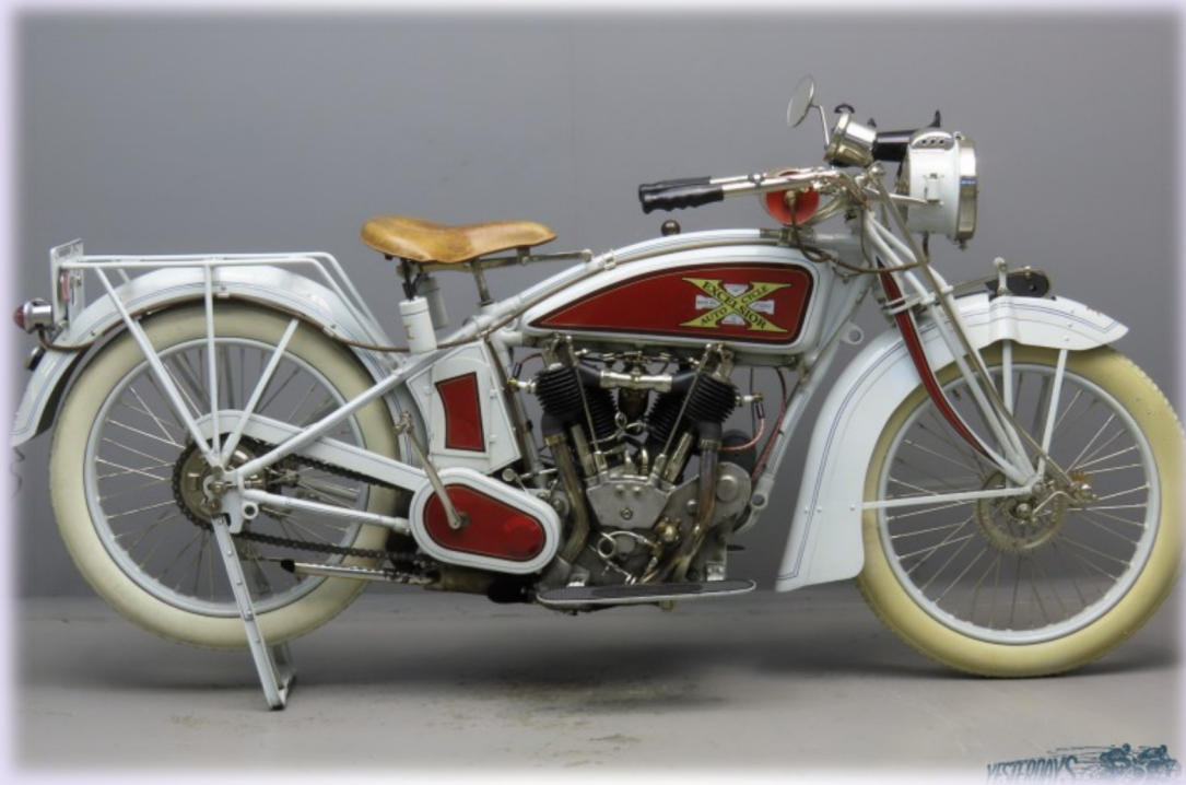
Excelsior 1919 "Series 19" 974cc (61 ci) IOE V-twin engine
