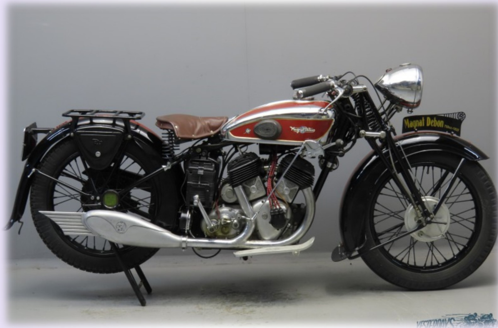
Magnat-Debon 1935 'VMA' 748cc side valve v-twin
