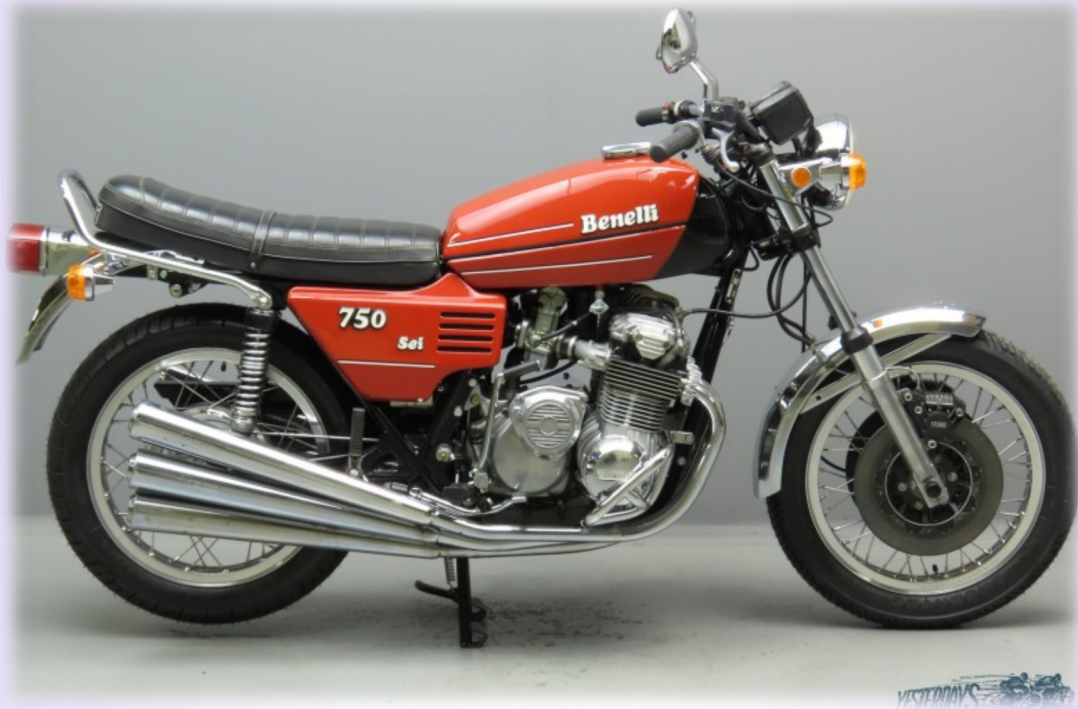
Benelli ca. 1977 "Sei" 748cc transverse six cylinder OHC
